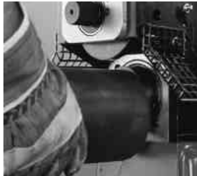
Fig 09: Lay pipe over roll.
