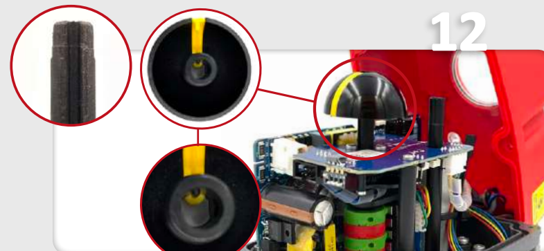
Carefully insert the position indicator, matching its inner key with the cleft of the shaft.
