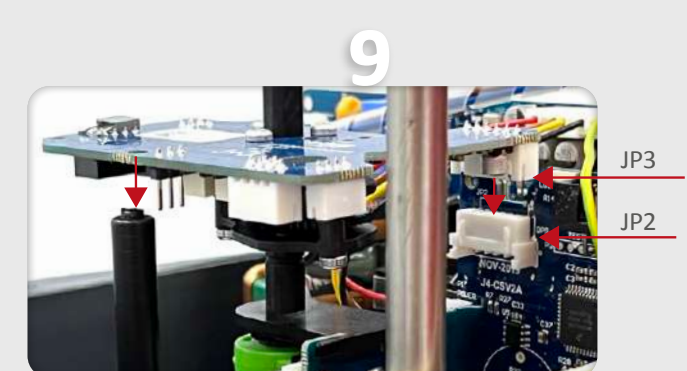
9 Press the DPS positioner PCB (Element C) along the shaft until the PCB connector (JP3) is plugged in the actuator PCB connector (JP2).
