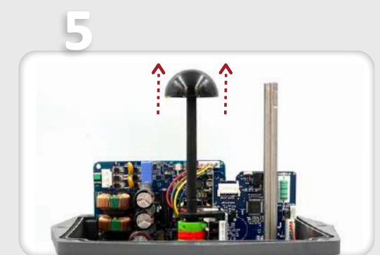
5 Carefully remove the position indicator.
