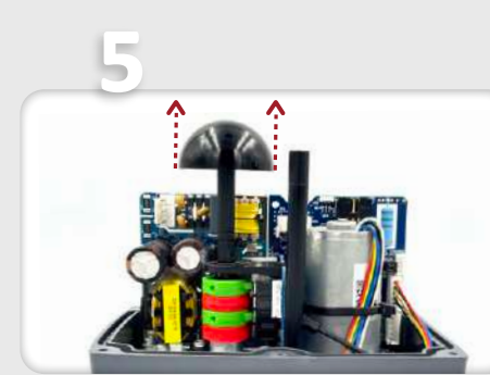
Carefully remove the position indicator.
