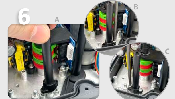
Fix the plastic column (Element B) on the base plate, by using 2 sheet metal fixing screws (Element D) (Fig. A, B and C).
