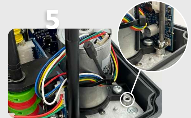
Fix it to the actuator metal plate, by using the Sheet metal fixing screw (Element E).
