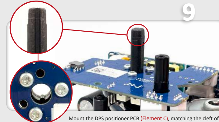
Mount the DPS positioner PCB (Element C), matching the cleft of the shaft with the key inside the DPS gear.
